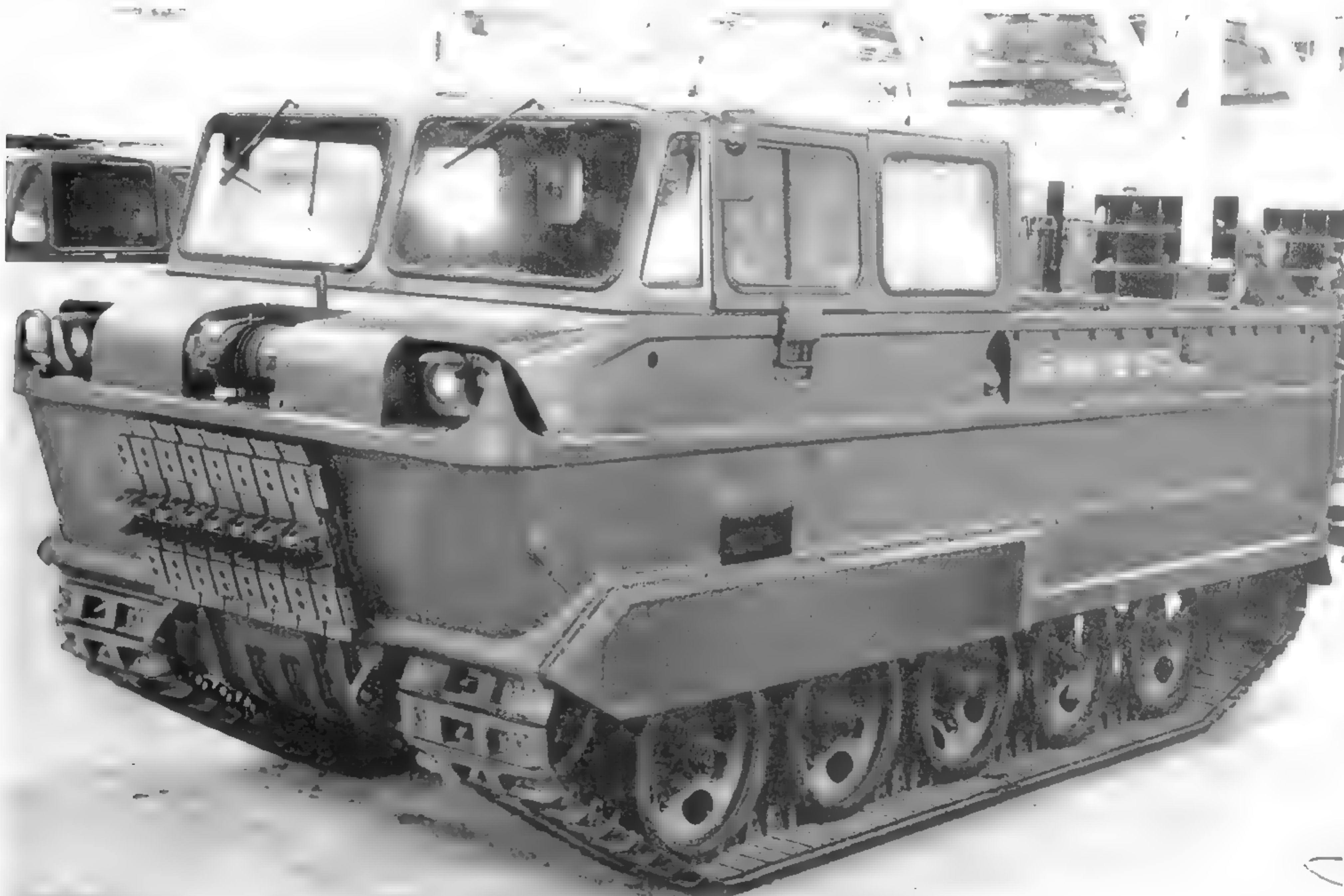
The M116 Husky was the answer to the Army's desire for a lightweight amphibious carrier. This vehicle was photographed in the Pacific Car and Foundry Company plant, and such details as the front-mounted winch found on all Huskies, and the wide track the provided superb flotation in snow, mud and sand.
